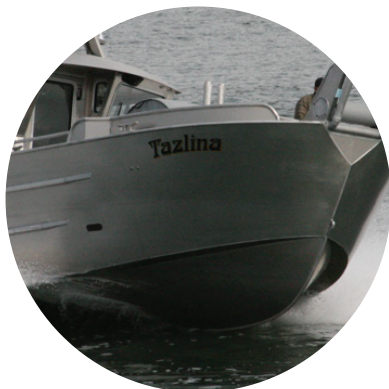
9.8M X 3.7M BOW PICKER 29 KNOTS @ 10,208KG DISPLACEMENT
